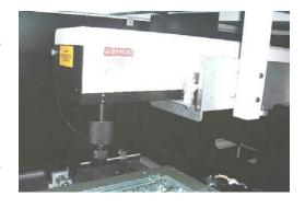
Laser Head delivers Laser Beam to spot weld the parts mount on the worktable
